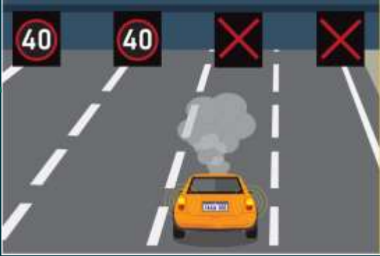
Variable Speed Limit & Temporary Use/Closure of Lane/Shoulder
